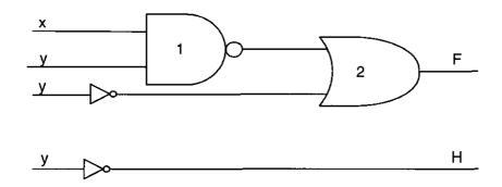
These two logic circuits are not equivalent F = (xy)' + y' and H = y' One of the two gates can be changed so that the circuits can become equivalent. Which gate can be changed and what kind of gate must it become?
