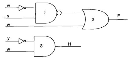
These two logic circuits are not equivalent F = (w'y)' + w and H = y'w One of the three gates can be changed so that the circuits can become equivalent Which gate can be changed and what kind of gate must it become?
