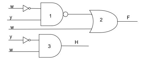
These two logic circuits are not equivalent. The outputs are  $F = (w' \cdot y)' + w$  and  $H = y' \cdot w$ . One of the four gates must be changed in order for the circuits to become equivalent. Which gate must be changed and what kind of gate must it become?
