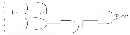
What is the final output T(x, y, z) of the given logic circuit?
